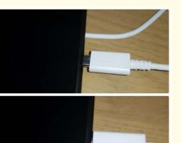
Gently push the smaller end of the cable into the hole in the bottom of the tablet. Make sure the little symbol is facing the top otherwise it won't go in.
