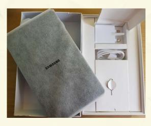
Open the tablet box, inside you will see a tablet, a charging plug, a charging cable & a little silver pin
