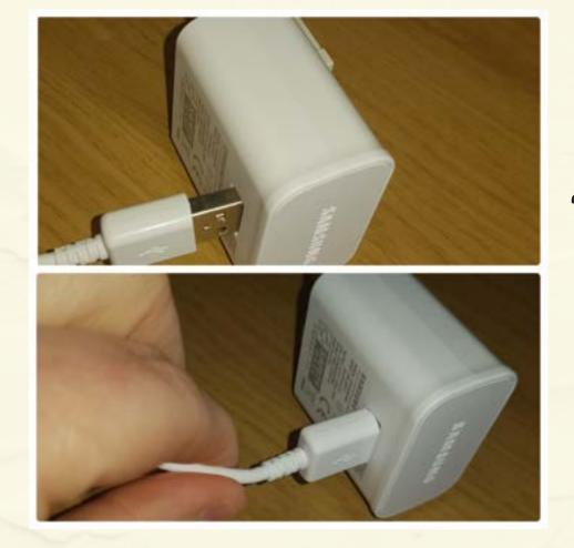
To insert the cable into the plug hold the cable with the little symbol facing to the side that has Samsung written at the top and gently push it in.
