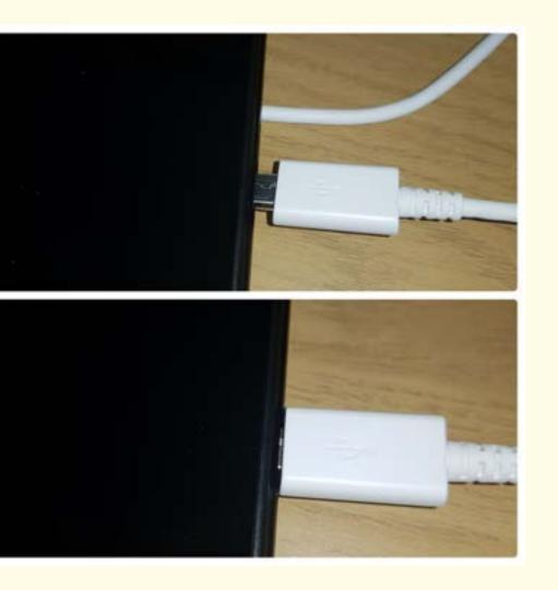
Gently push the smaller end of the cable into the hole in the bottom of the tablet. Make sure the little symbol is facing the top otherwise it won't go in.
